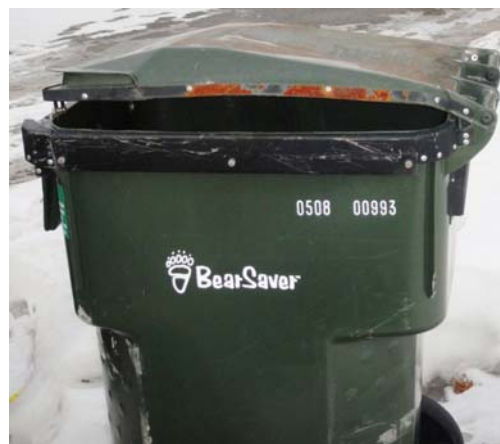
Figure 15: BearSaver compost cart at Yukon College showing the damaged lock mechanism which has been sprung by excessive force during the process of emptying.
