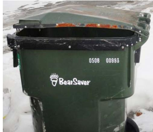
**Figure 15:** BearSaver compost cart at Yukon College showing the damaged lock mechanism which has been sprung by excessive force during the process of emptying.
