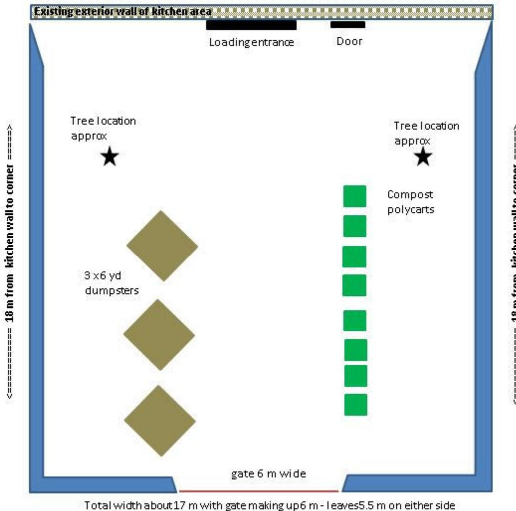
**Figure 10:** Sketch showing the location of a proposed electric bear fence at the Yukon College kitchen service area to provide a bear-proof “corral” to store regular garbage dumpsters and regular compost carts. The fence would be located in the solid blue area on 3 sides and meet against the existing wall.
